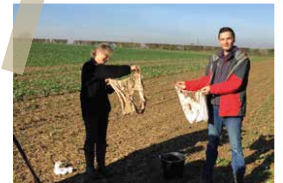
Fig 2b: University of Lincoln staff demonstrating the underpants test – high decomposition (left) and low decomposition (right) after burying in different soil environments
