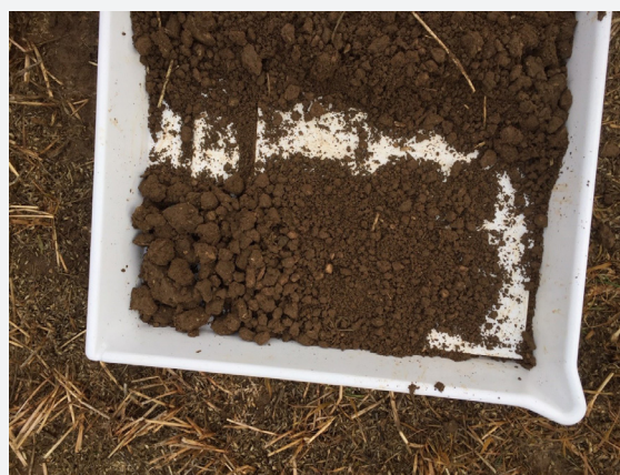
Fig 1a: Soil aggregate size distribution following VSA breakdown
