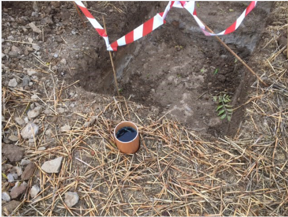
Fig 1c: Soil pipe infiltration test
